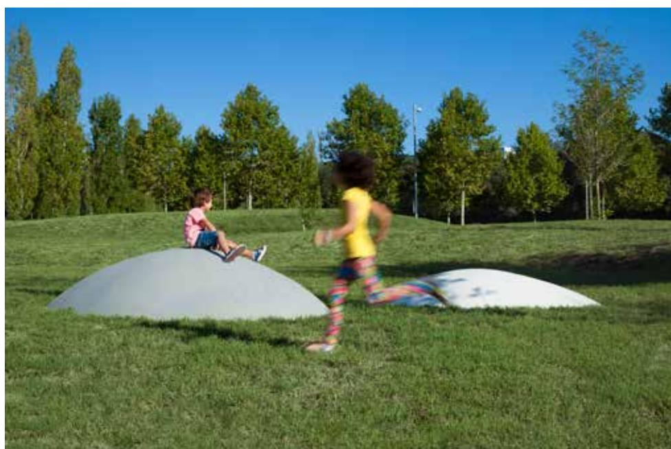
EN - UHPC concrete landscape element colored in mass, acid etched and waterproofed.
