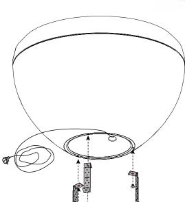
**3 X COUNTERSUNK SCREWS** M 10 mm - 16 mm
